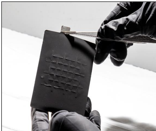
The pre-defined slit pattern on the electrode breaks into smaller electrodes, each too small to ignite thermal runaway.
